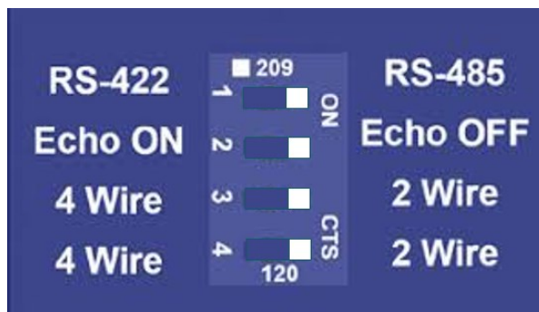
Figure 15: Dip Switch settings
