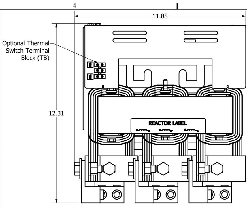
See V1K Installation Guide For Terminal Wire Size And Torque Information.
