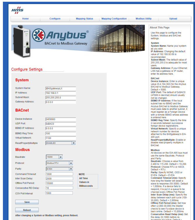
Figure 9.25: BACnet Gateway Configuration Page
