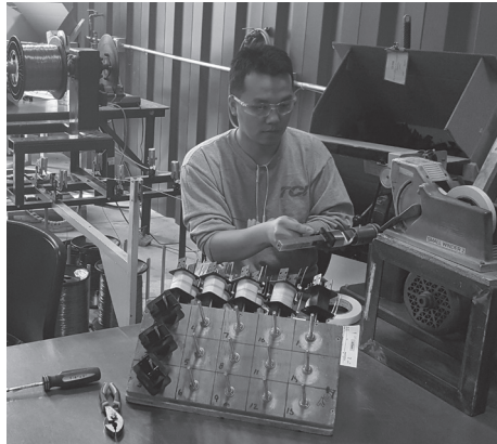
Operators in a cell wind coil for small line reactors.
