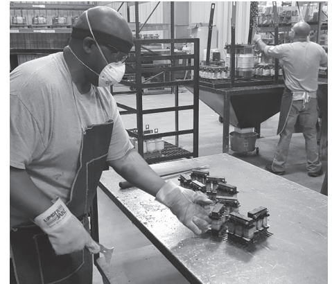
Small line reactors in their final stage: varnish, bake and clean.
