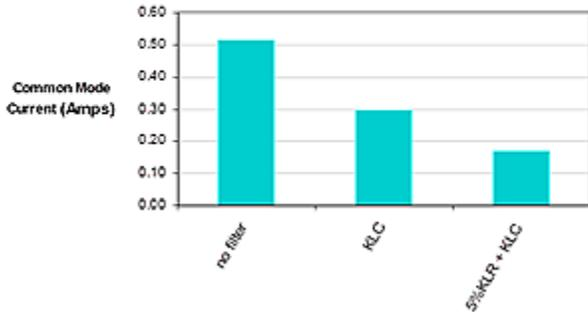
change of the PWM switching increases the capacitive coupling impedance between bearings and bearing races. The increase in capacitive coupling, in turn, reduces the damaging Common Mode Currents and increases motor up-time.
